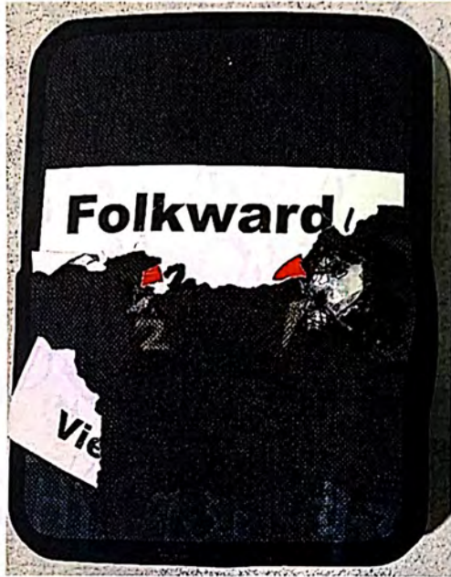
Fig. 1 Bulletproof Plate-ECO Sideplate 15×20 (strike face)
