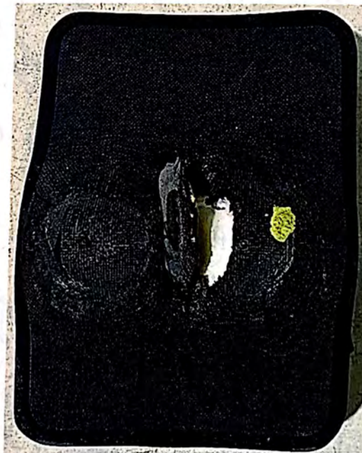
Fig. 2 Bulletproof Plate-ECO Sideplate 15×20 (wear face)
